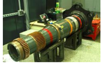
Completed Ferrium C61 CH-47 Chinook Forward Rotor Shaft
