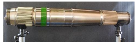
Sikorsky's MH-60S Helicopter Mast produced from Ferrium S53
