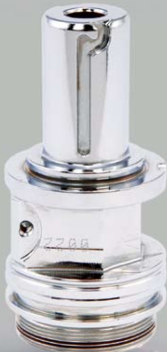
Stricter emissions requirements translate into much higher pressures, which means the steel used for fuel-injection systems, for example, must have higher toughness and better fatigue characteristics. Shown is a diesel fuel injector body manufactured from parapremium carburizing steel supplied by Timken.
