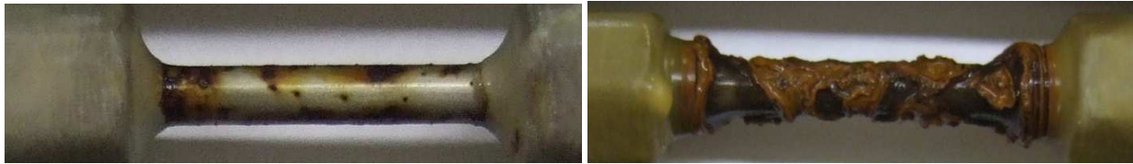
Figure 4 Final results of Ferrium S53 at 220 ksi (left) vs. 300M at 130 ksi (right) tension-loaded specimens in ASTM G49 test, alternately submerged in 3.5% NaCl solution and air for 1,000 hours.
