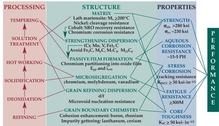
Performance requirements for commercial and defense aircraft have always required high specific-strength materials for critical landing gear components. Until recently, designers had to compromise between strength and corrosion resistance: They had to choose between steels such as 300M, 4340, and AerMet 100 for ultra-high strength but relatively low corrosion resistance; or stainless steels such as 17-4 and 15-5, which provide higher corrosion resistance but less strength.
