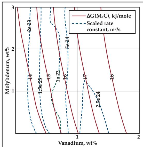
Fig. 2— Calculated overall precipitation driving force and coarsening rate constant.
