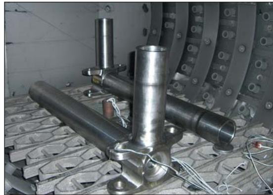
Fig. 3 — A-10 MLG pistons in heat-treatment. Image courtesy Solar Atmospheres.
