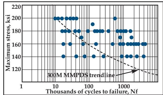
Fig. 4 — Longitudinal and transverse S53 axial fatigue data vs. 300M, R = -0.33.
