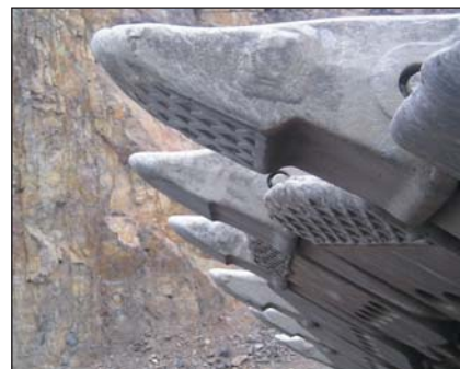
Left, a TEM micrograph shows the nanometer-size grain structure of one of NanoSteel's SHS alloys. Right, the SHS hardfacing applied to the excavator bucket tooth in the foreground provides a sharp contrast in wear protection when compared to bucket teeth in the background which have not been hardfaced.
