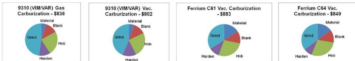
Figure 14. Distribution of gear production costs for manufacture of a high-performance aerospace gear using different carburization techniques and materials
