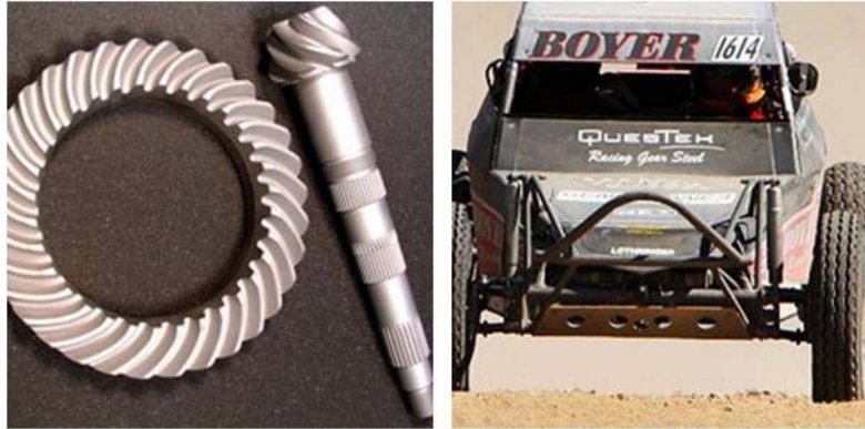
Figure 9. Example of ring gear (left) in a high-performance off-road racing application used in 1/-1600 SCORE series
